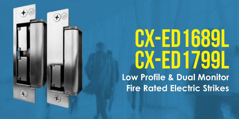
**Camden CX-ED1689L** and **CX-ED1799L** Grade 1 electric strikes for mortise and cylindrical locksets offer the very best strike quality and features, with the added value of built-in single or dual latch monitoring, 4 or 8 stainless steel faceplates and 'Universal' performance, including field selectable voltage and fail safe/fail secure operation. These strikes also include a 3-hour fire rating, and also have the option of ordering strike bodies and individual faceplates separately.
